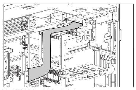
Figure 2-25. Diskette drive cable folding and routing diagram
